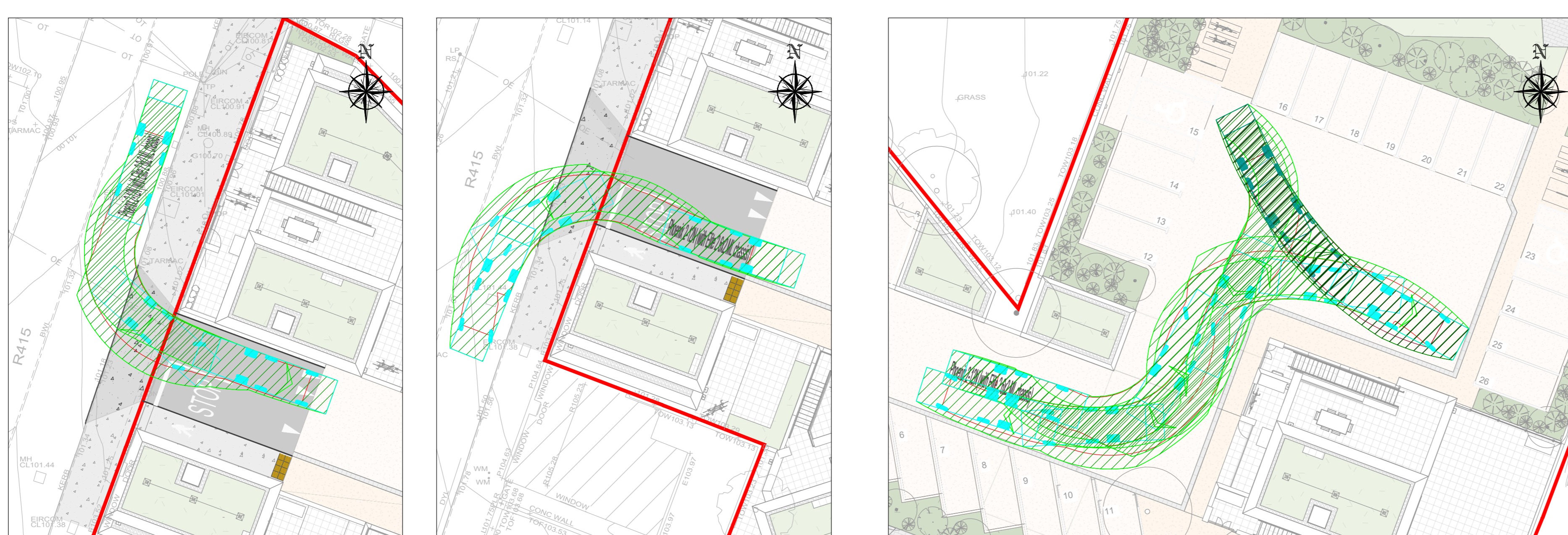
REFUSE VEHICLE SWEEP PATH. SCALE 1:200
